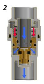
EASYRID, is the simplest pressure reducing valve of ever. When all users are closed, the pressure inlet strenght (blue arrows) helps the valve to close the water passage. Is enough open just one user, to decrease the pressure and in this case the spring (red arrows), designed for get 3/3.5 bar pressure outlet, is able to open the valve and to allow the passage of water.
